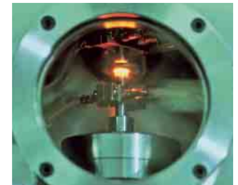
Solidifying cycle weld simulator
