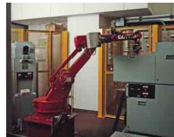
Radiographic film processor (robot)
