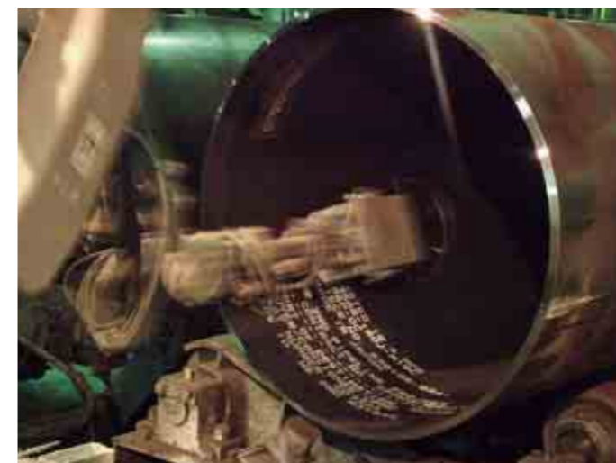
Automatic pipe marking
