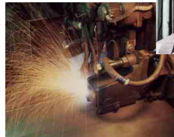
Continuous CO 2 tack welding
