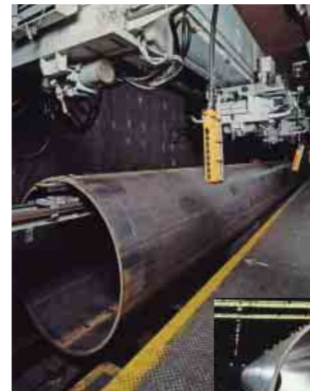
Full length X-ray radiographic examination system
