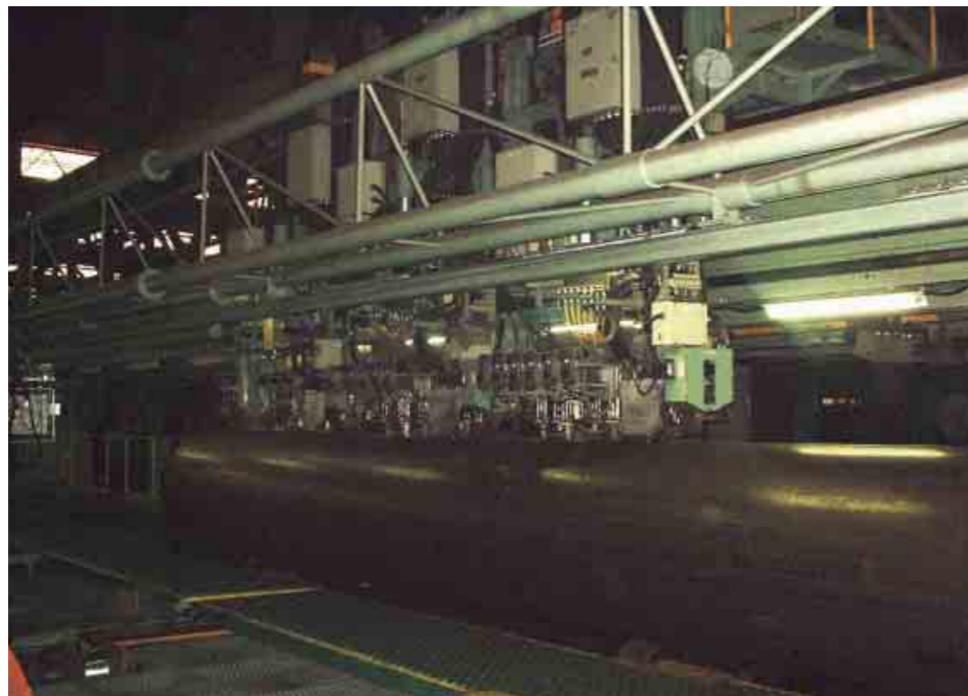
Automatic UST of weld
