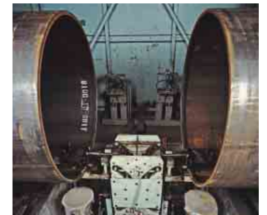
Pipe-end X-ray radiographic examination system
