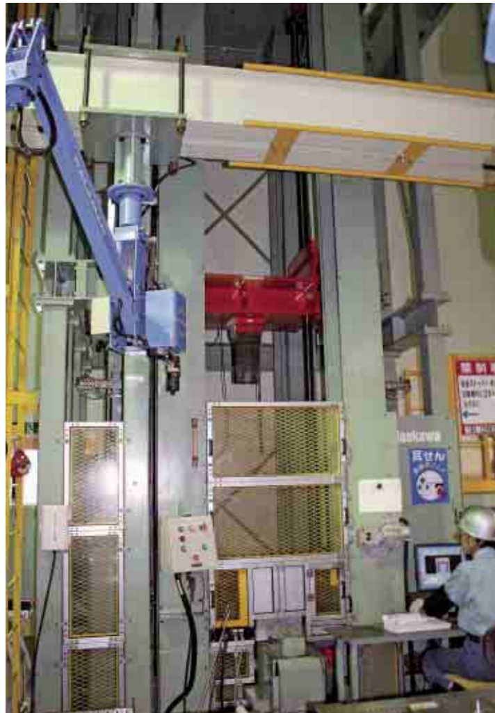
Drop Weight Tear Test (DWTT)
