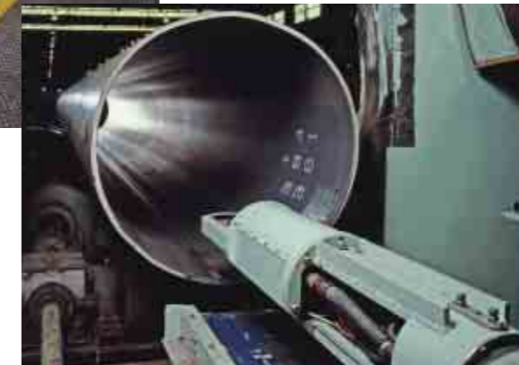
X-ray fluoroscopic examination system
